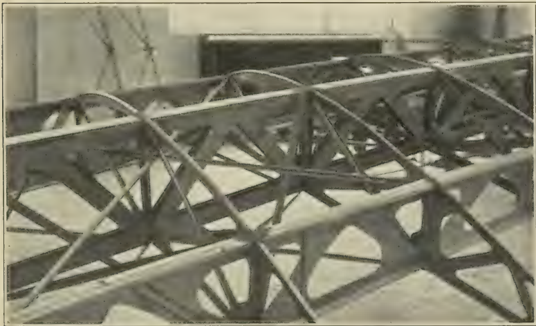
2.—ELABORATE INTERNAL TRUSSWORK OF A GLIDER WING
